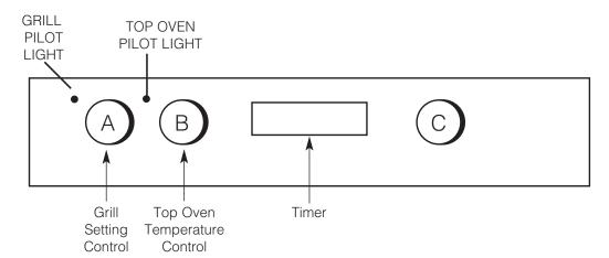
Step 1 Ensure oven timer is set to manual. Place the shelf in the correct position (see Grilling Guide). Place the food/grill pan on the shelf, positioned centrally under the grill element. Leave the top oven door fully
